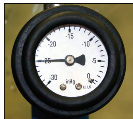
Pump Gauge Holding 25 inHg of Vacuum
