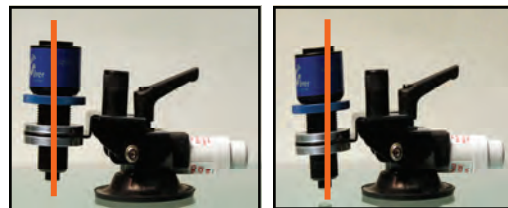
Before and After Canting the Fixture
