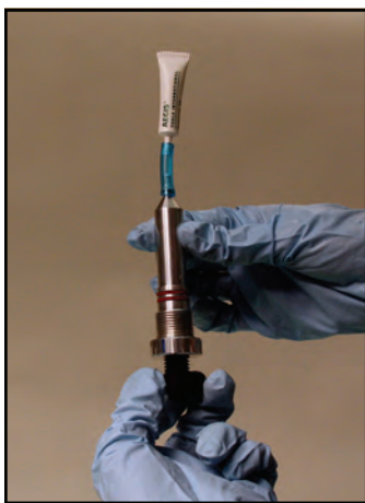
Drawing resin into the adaptor and injector
