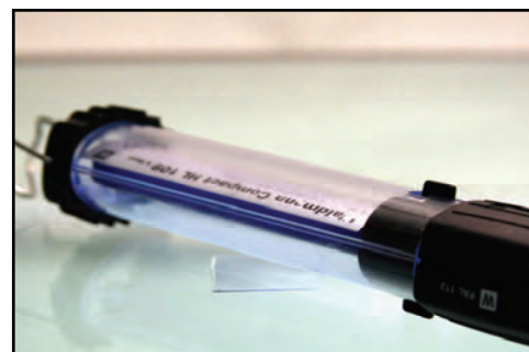
Curing the Resin (110 V UV Lamp (LMP3500) shown)
